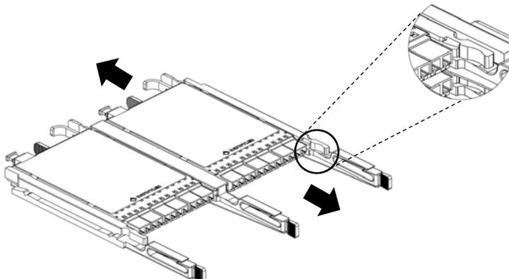
Each sliding tray can be installed with 2 cassettes
