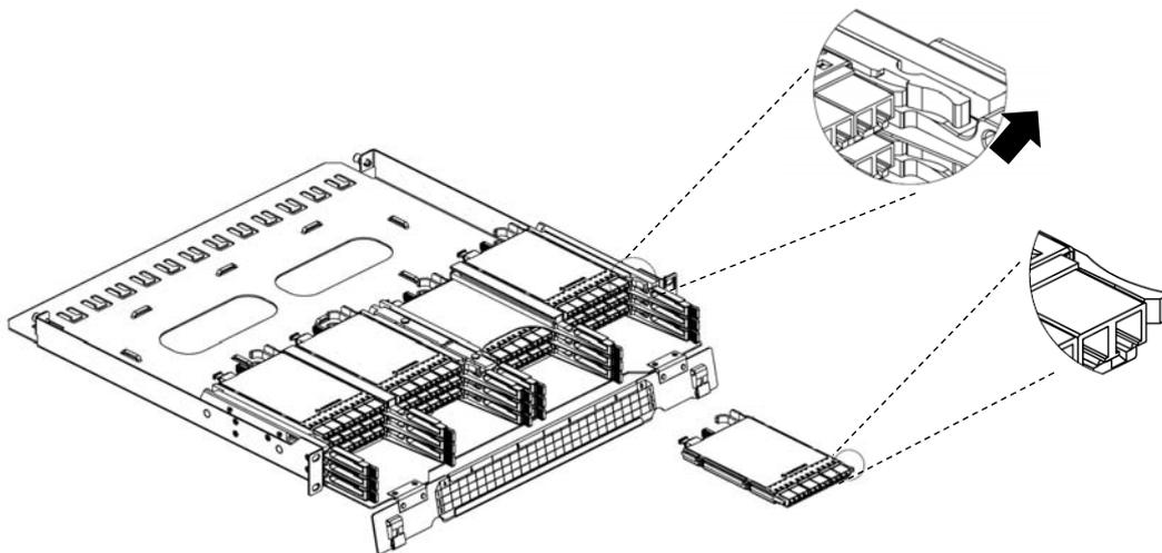
There is a fixation point as shown which can fix the cassette to avoid dropping
