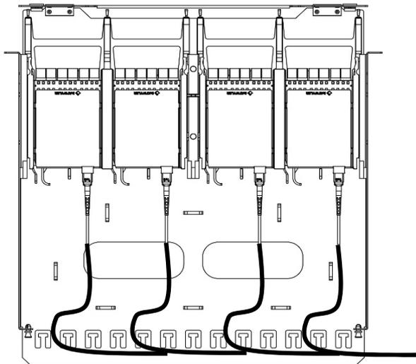
The fibres can be routed as shown or according to actual situation
