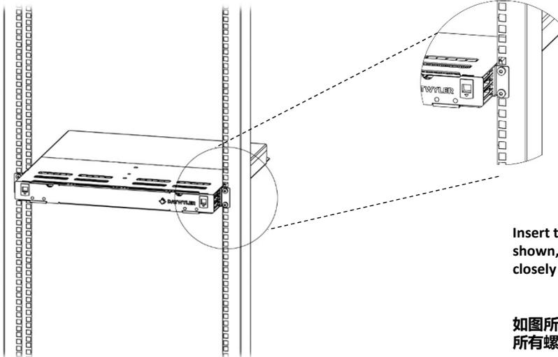
Insert the screws ( provided ) into the desired holes as shown, tighten all screws and ensure the panel be fixed closely
