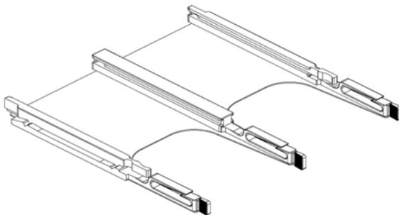
Each sliding tray can be pushed, pulled and removed with the tab from front side
