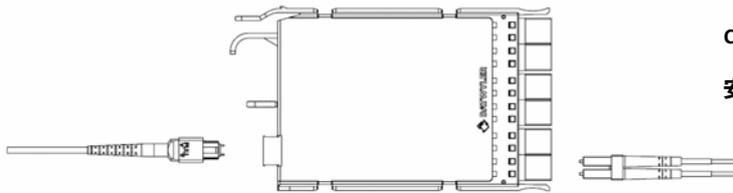
Clean MTP/LC adapter and connector before installation
